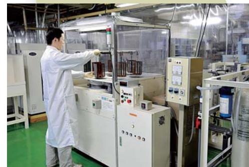
密封循环电泳装置 Electrodeposition closed system
