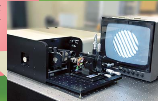
微光学系统开发与事例：微粒子监测器 Example of micro-optical system development: Particle monitor
